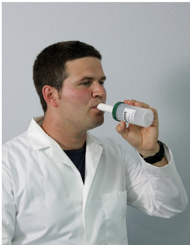
Fig. 5. Bio-VOC breath sampler (Markes International Ltd., UK) developed by UK HSL.
