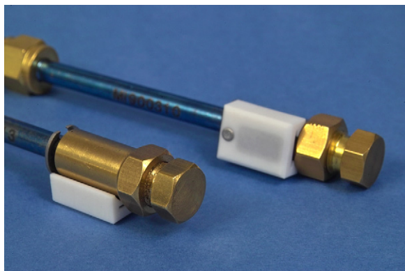
Fig. 3. RFID tags attached to thermal desorption sorbent tubes.
