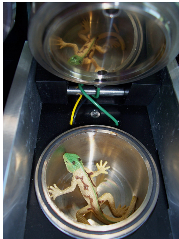
Fig. 4. Child's plastic toy inside a micro-chamber prior to analysis. (a) Schematic of a single micro-chamber as used for bulk emission testing.
